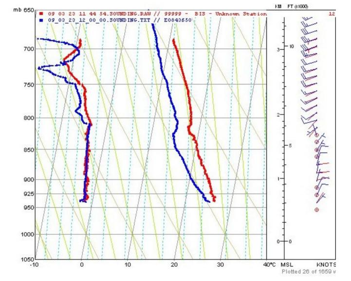
Comparison between the AIMMS measurements (red) and the Riyadh rawinsonde sounding on 23 March 2009. Additional analysis shows that typically the AIMMS probe temperature was greater than the Rosemount temperature and greater than the temperature measured by rawinsonde. The Rosemount temperature probe is a more robust measurement.
