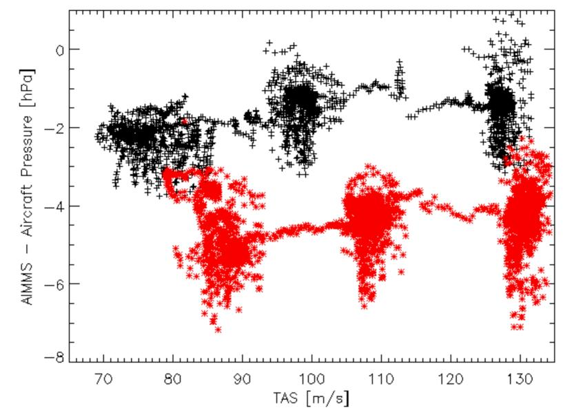
The difference between the Aircraft Integrated Meteorological Measurement System (AIMMS) measured pressure and the pressure measured at the aircraft's static pressure port during the 23 March 2009 aircraft flight in Saudi Arabia. The black plus samples are at 15,000 ft sampling and the red starts at 21,000 ft.
