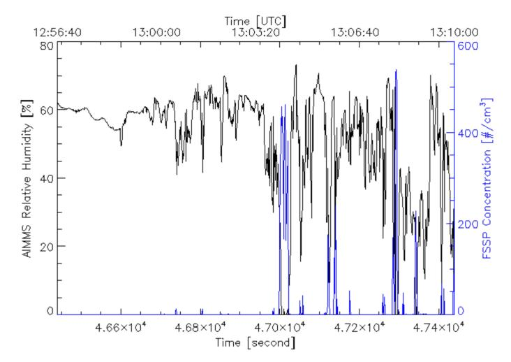
Time series showing the AIMMS relative humidity (black trace) and the FSSP cloud droplet concentration (blue trace) during the 8 April 2009 flight in Saudi Arabia. This time series is during the beginning of the flight just after the aircraft reached a constant flight altitude of 4500 m (temperature of approximately -4 C). As indicated by the FSSP cloud droplet concentration, at approximately 47000 seconds the aircraft first penetrated a cloud.
