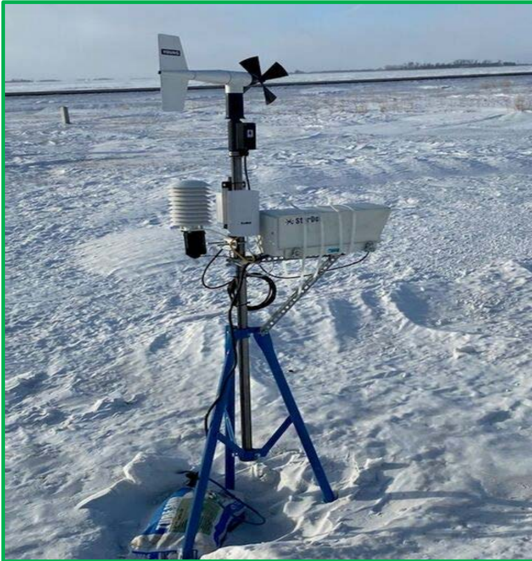
Figure 5. A picture showing the ground-based tripod system. The IMet-XQ2 is located in black underneath the radiation sensor on the left side. The Young Anemometer is located at the top of the tripod. The MiniOFS is located at the front of the camera box, outside of view. Power to the system is supplied by Ice Crystal Engineering Headquarters through extension cords.
