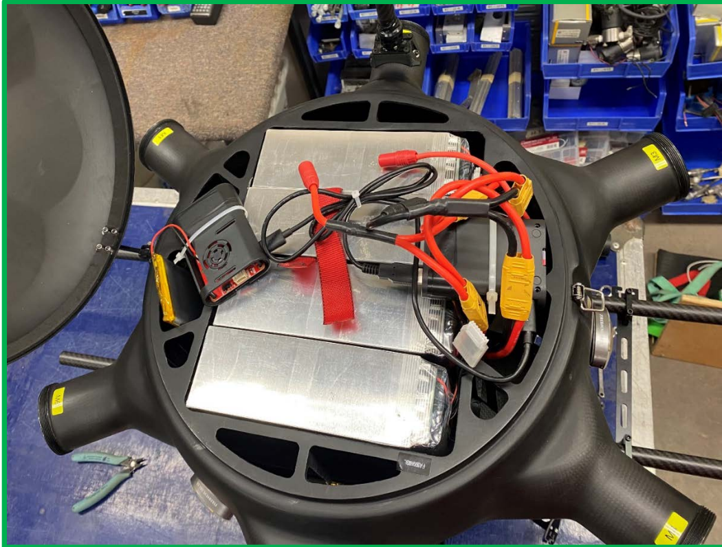
Figure 4. A picture showing the internal body of the Unmanned Aircraft Vehicle (UAV). The four lithium-ion batteries are displayed in silver, with the internal instrumentation/electrical components placed on top for image visualization. Normally, the internal wiring/electrical components are stored within the gaps of the UAV frame around the lithium-ion batteries.
