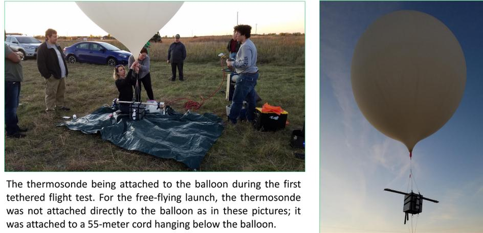
The thermosonde being attached to the balloon during the first tethered flight test. For the free-flying launch, the thermosonde was not attached directly to the balloon as in these pictures; it was attached to a 55-meter cord hanging below the balloon.
