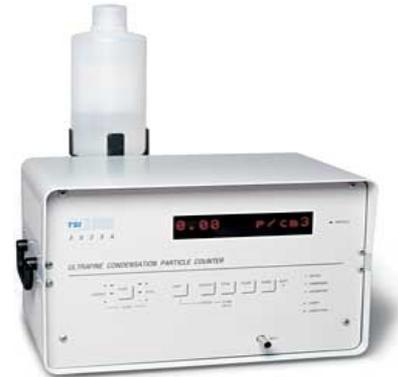
Alcohol vapor condenses onto particles which create droplets large enough to be detected one at a time by an optical particle counter. Upon entering the instrument, the air sample passes through a saturation block where alcohol evaporates saturating the flow. The air sample next enters a condenser tube which cools the air sample. Cooling of the air sample creates a supersaturated environment and the alcohol condenses onto particles, regardless of particle composition.
