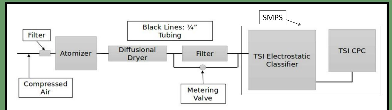
Image showing the instrument setup for obtaining the size distribution of the liquid smoke using the TSI Scanning Mobility Particle Sizer (SMPS) which is the combination of the TSI Electrostatic Classifier and the TSI Cloud Condensation Particle Counter (CPC).
