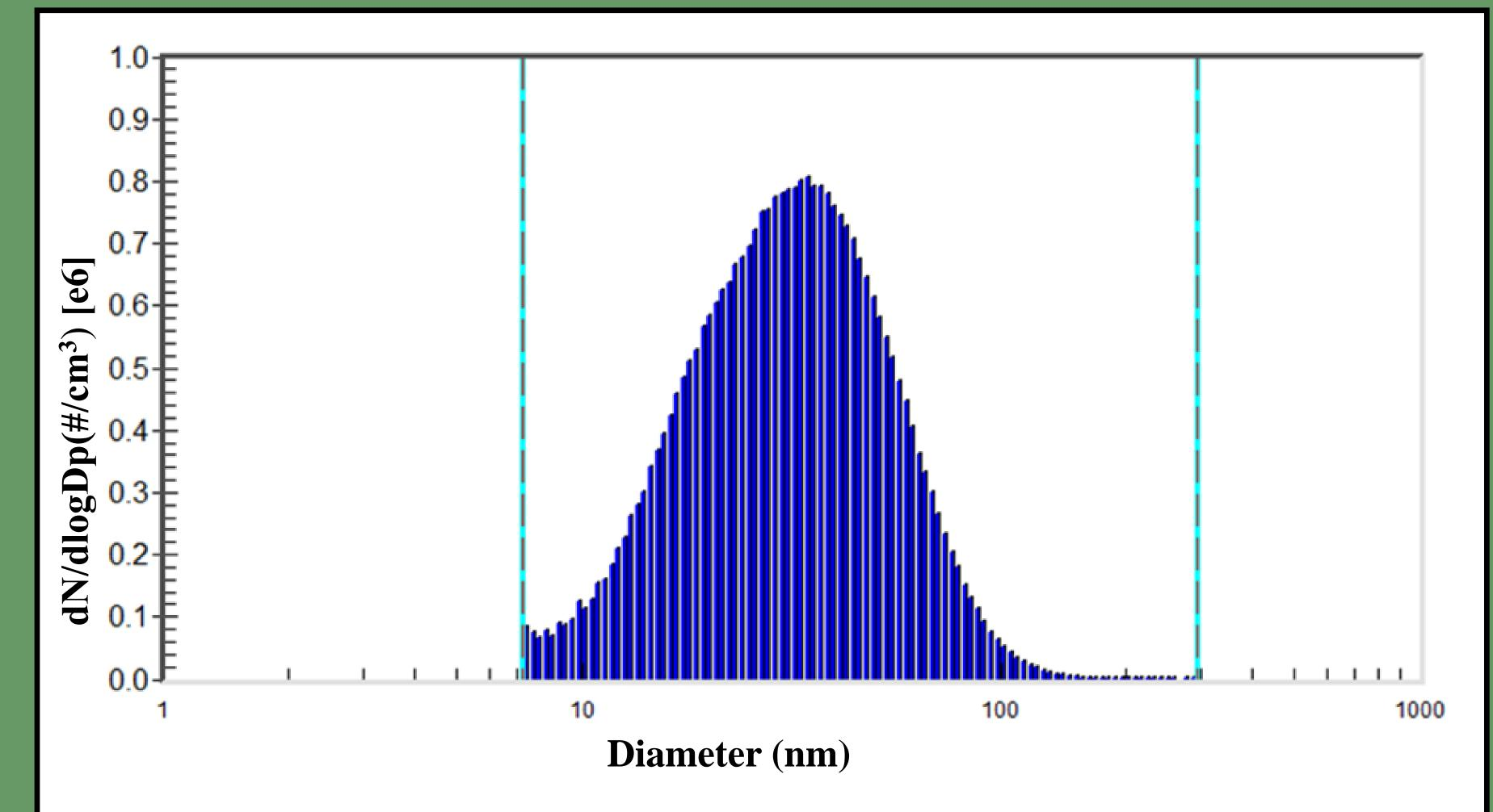
Scanning Mobility Particle Sizer (SMPS) measurements of a solution of 0.03 % liquid smoke and ultra-purified water.
