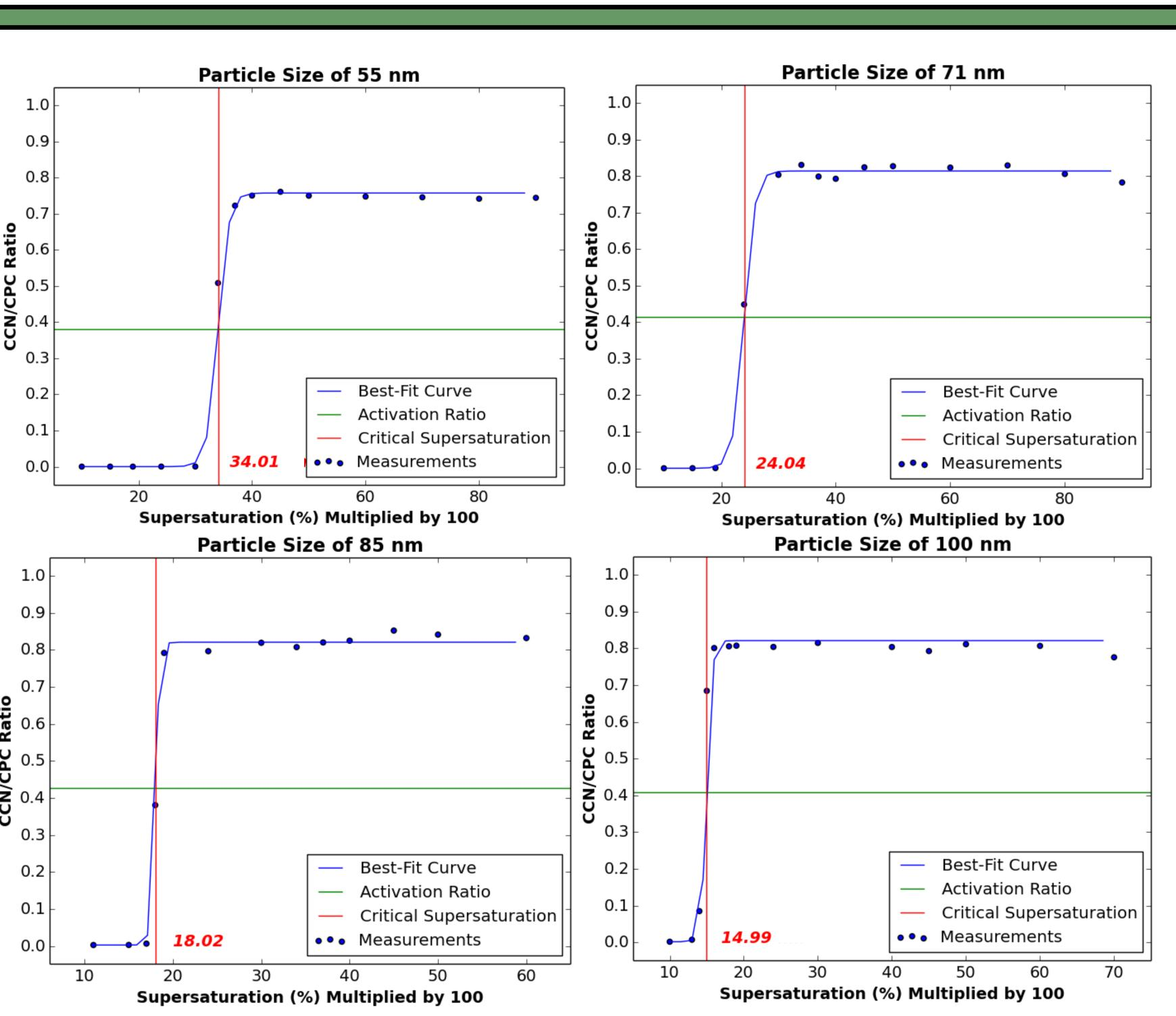
Activation Curves to find the Critical Supersaturations of 55, 71, 85, and 100 nm size particles of Liquid Smoke. Data taken using lab set up in upper right panel. Critical supersaturations are indicated in red and used to calculate Kappa.
