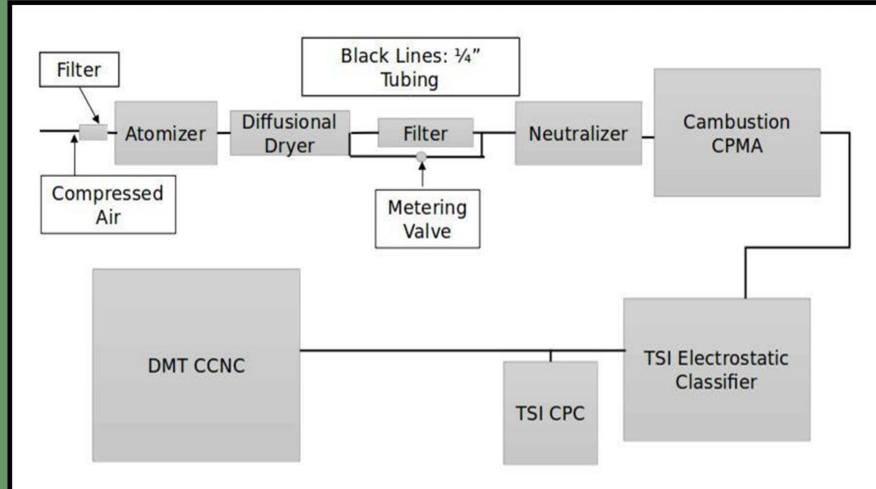
Image showing the instrument setup for finding the Kappa values of liquid smoke using the Centrifugal Particle Mass Analyzer (CPMA), TSI Electrostatic Classifier, CPC, and the DMT Cloud Condensation Nuclei Counter (CCNC).
