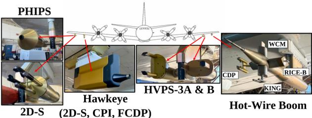
Fig. 1 Schematic of the NASA P-3b Research Aircraft and the instruments installed under the wings of the aircraft.
