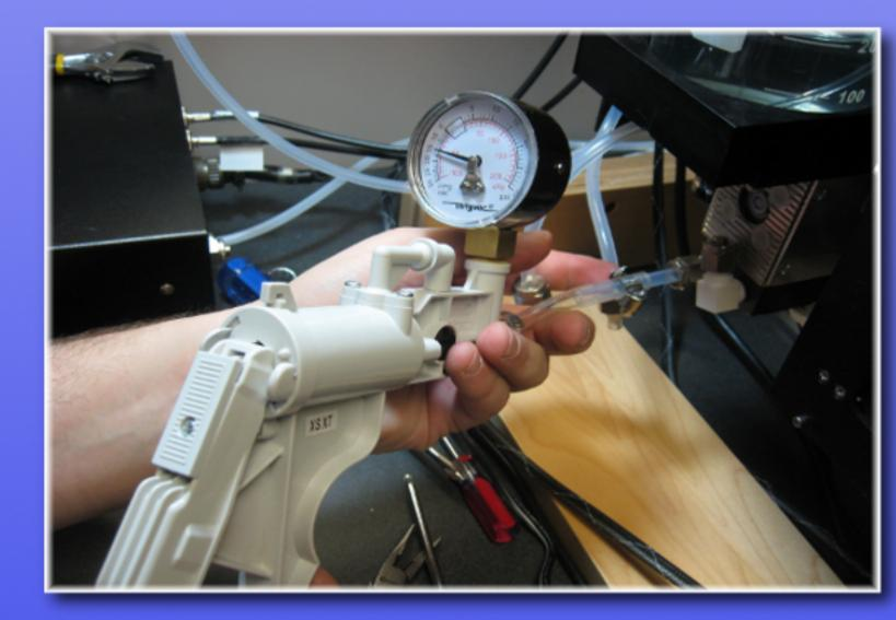
Sheath flow calibration was performed using a manual flow meter setup. Due to this process' being lengthy and error-prone, in the future this setup will be replaced with an automatic flow calibrator system. (Sensidyne Gilian Gilibrator II)
