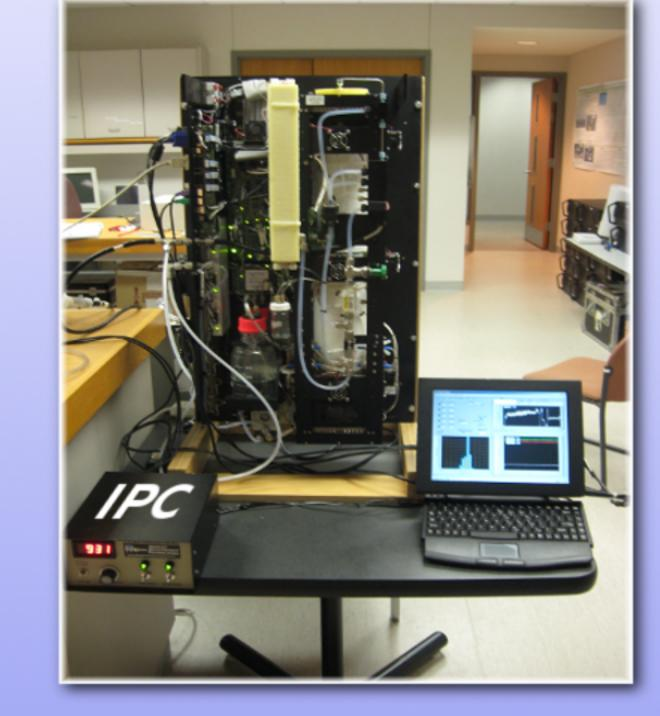
A general view from the experiment setup. Ammonium Sulfate aerosol particles were distributed into a DMT - Passive Cavity Aerosol Spectrometer Probe (PCASP), and TSI - Condensation Particle Counter (CPC) as well, to ensure the integrity of the experiments.
