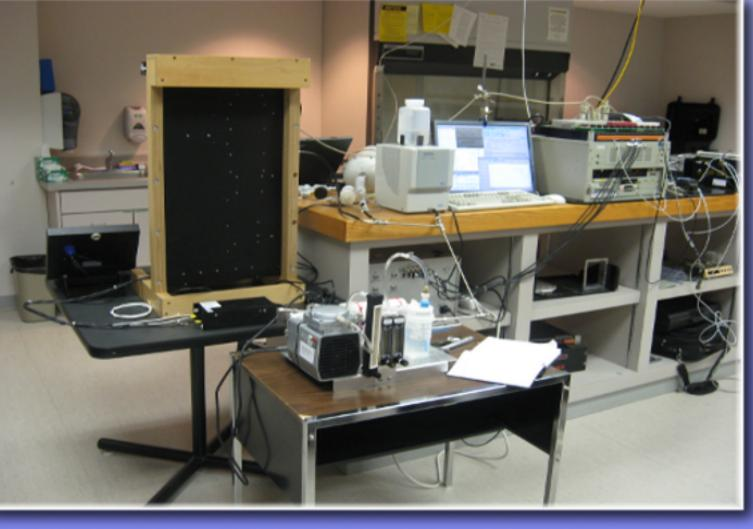
A handy leak tester is in action. Leak testing carries a great importance in order to obtain reliable measurements using a DMT-CCNC.
