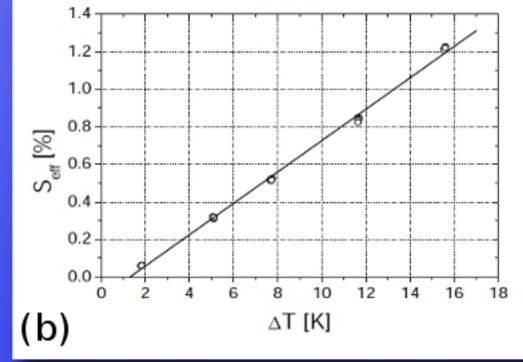
Example calibration experiment results with ammonium sulfate aerosol. (a) CCN efficiency spectra, (b) calibration line of Seff vs.  $\Delta T$ . (Mainz, 21 December 2005, Q=0.5 L/min, p=1026 hPa, T1=298.5 K) (Figures and data are from D. Rose et al.)
