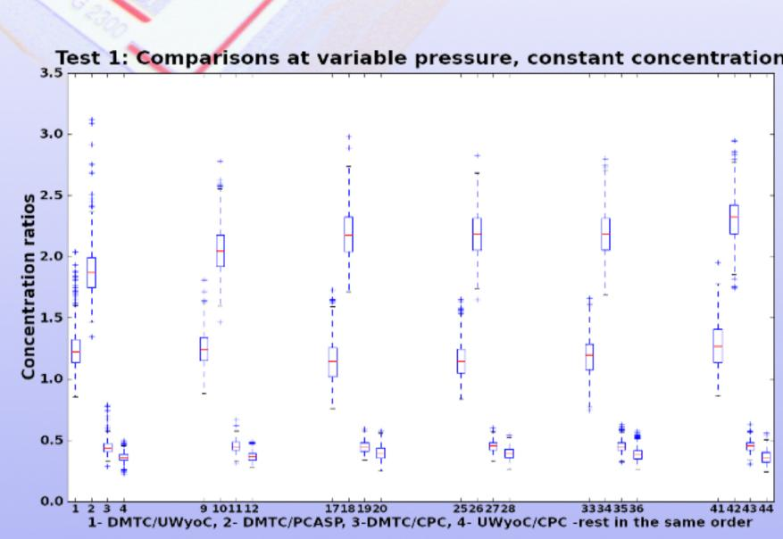
In the first leg of these experiments, while the DMT-CCNC's pressure being varied from 460 to 950 mB at six steps, aerosol concentration was adjusted to 600 #/cm^3 level based on the UWyo-CCNC readings. For this case and the following two cases, nine minutes long portion of the acquired data were analysed. The left figure shows the change of concentrations throughout each nine minutes intervals in four counters, whereas the right figure depicts the relations of the instruments with eachother.
