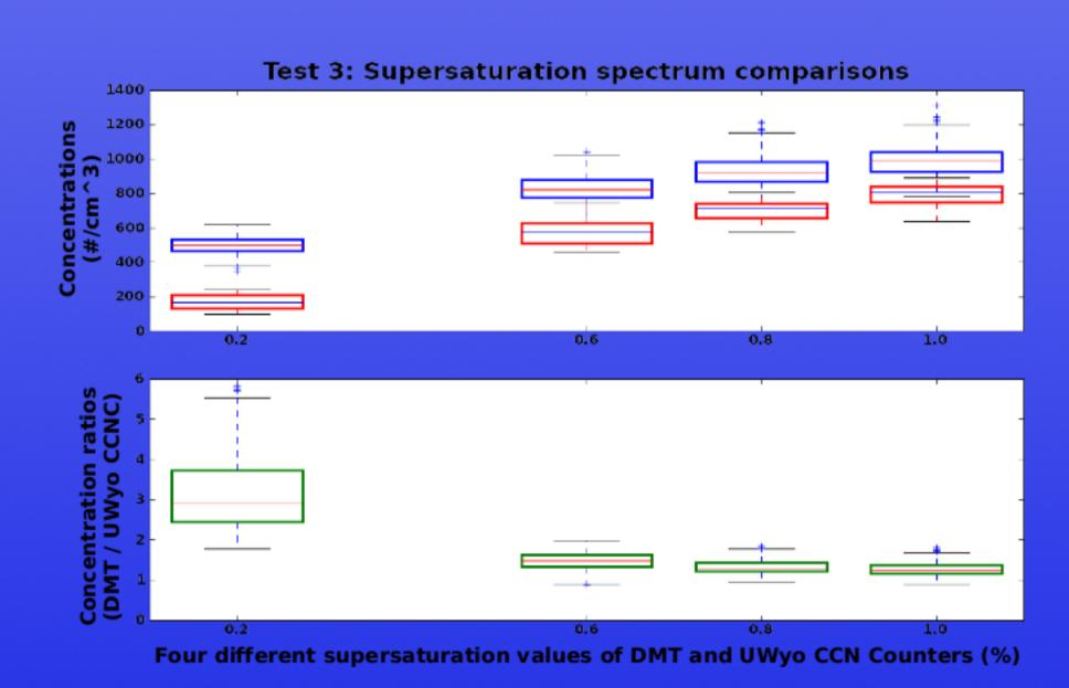
In the last experiment, both the DMT and UWyo CCNC measurement responses tested at 0.2, 0.6, 0.8 and 1.0 supersaturation settings, while DMT-CCNC inlet pressure was constant at 500 mB.
