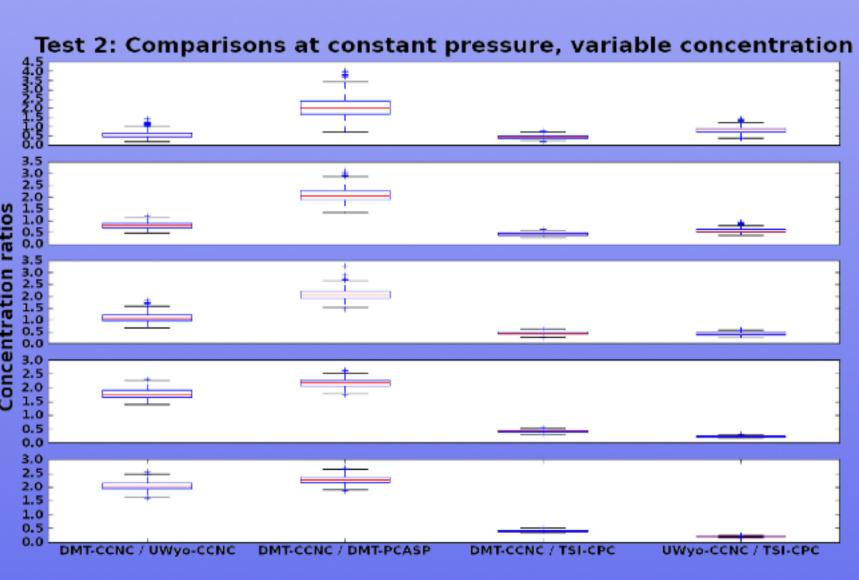
In the second test, the DMT-CCNC inlet pressure value was hold constant at 500 mB, UWyo-CCNC concentration readings changed from 150 #/cm^3 to 1800 #/cm^3 at five steps. Corresponding concentration outputs of rational comparison of each instrument are given on the left, and right figures, respectively.
