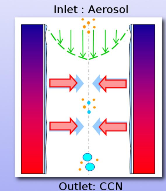
CCN measurements in Cylindrical Continuous-Flow Streamwise Thermal Gradient
