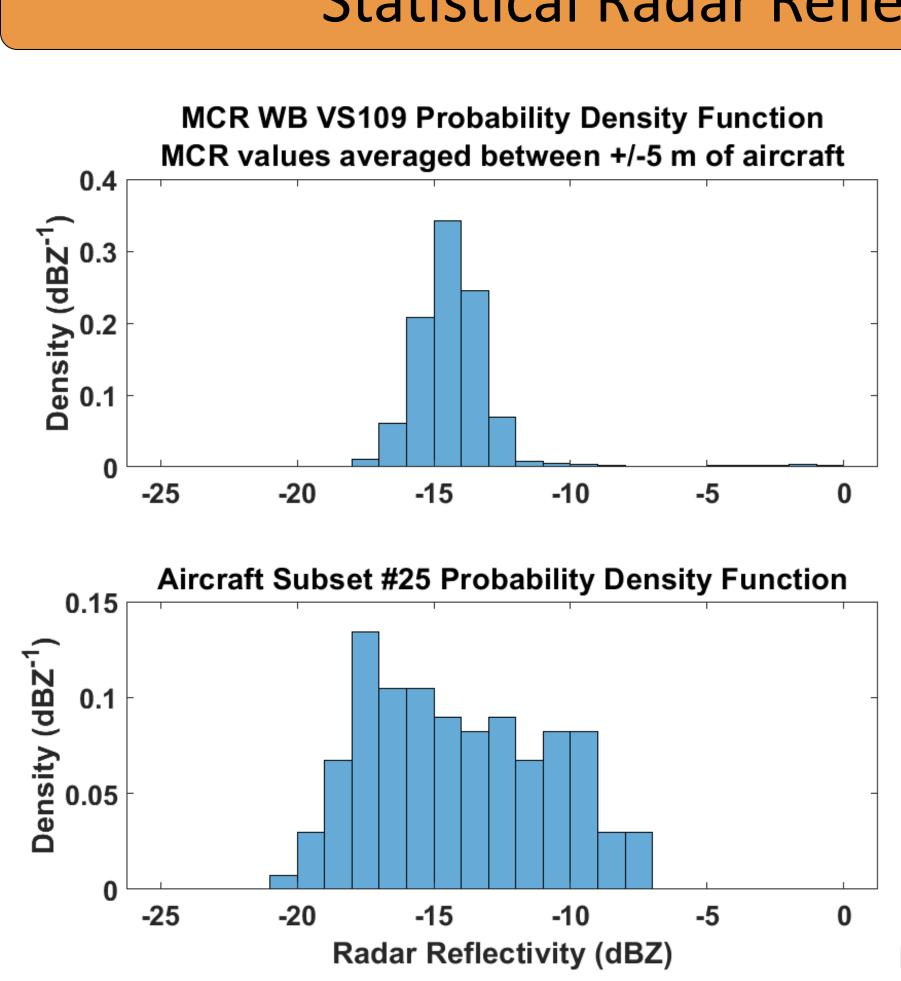
The probability density function of the narrowband reflectivity values (top) compared to the probability density function of the derived aircraft radar reflectivity values (bottom) from 17:37:42-17:40:05 UTC.. Good agreement exists between the MCR and derived aircraft radar reflectivity, but there is more variability in derived radar reflectivity data.
