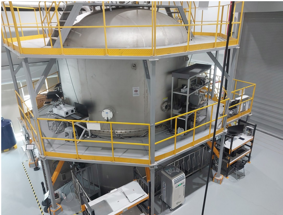
NIMS Cloud Chamber, Expansion Types, Volume 29.3 \text{ m}^3
