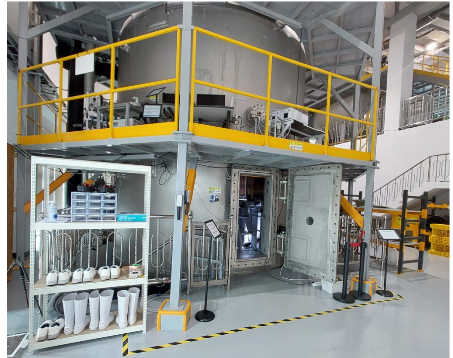
NIMS Cloud Chamber, Expansion Types, Volume 29.3 \text{ m}^3
