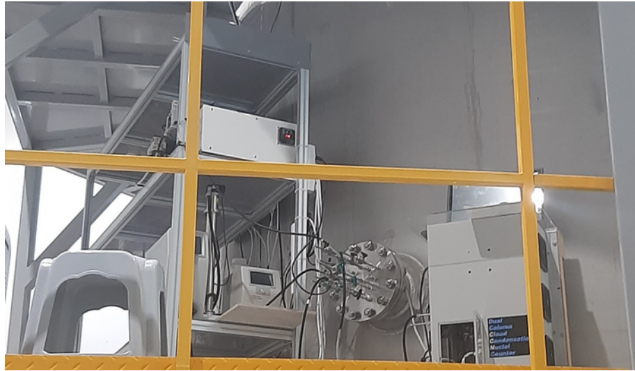
NIMS Cloud Chamber Expansion Types, Volume 29.3 m 3
