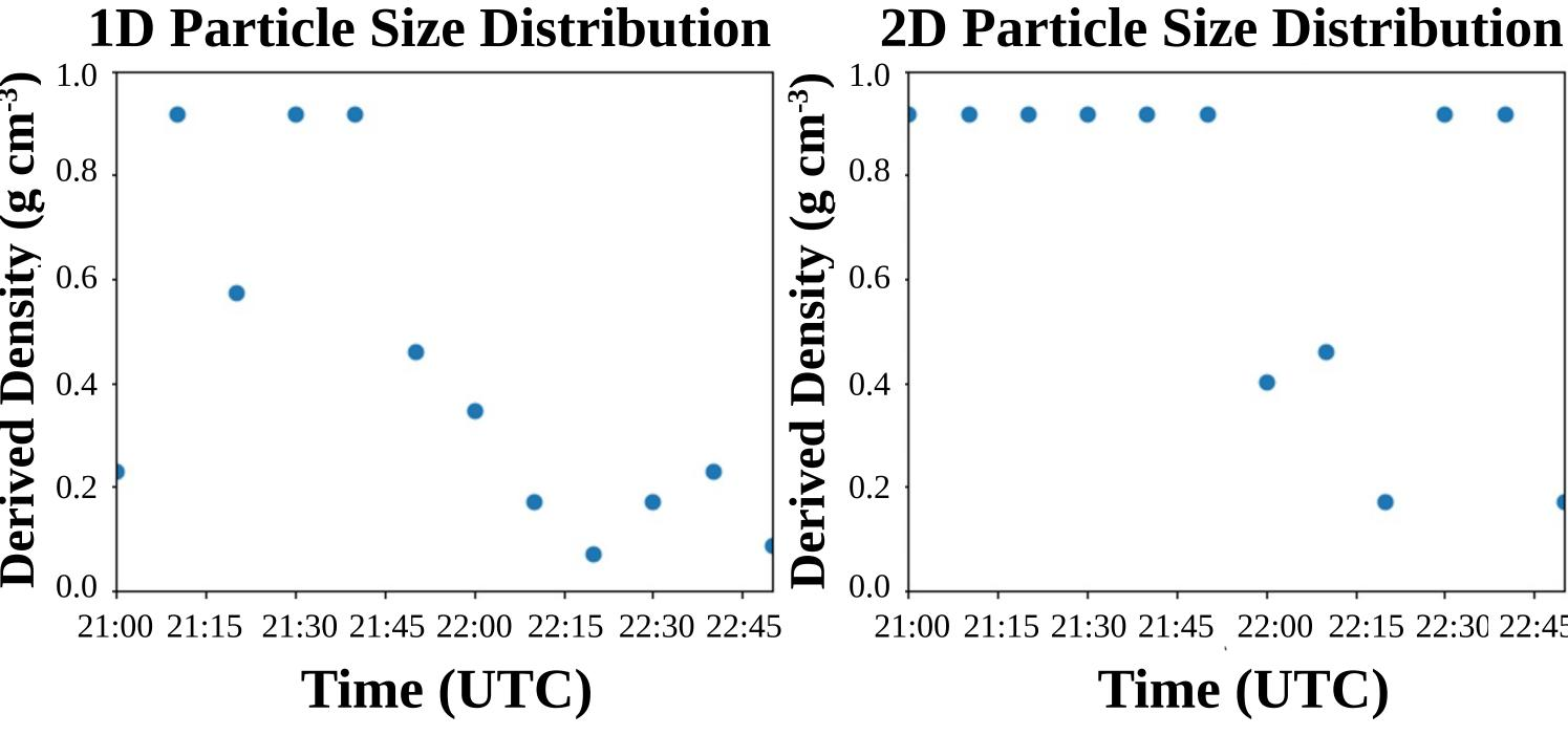
Derived particle densities used T-matrix calculations and matching the Hail Spectrometer particle size distributions during Flight 757 (24:21:00-24:23:00 UTC). The particle air fraction is used to obtain the best agreement between computed and observed reflectivities
