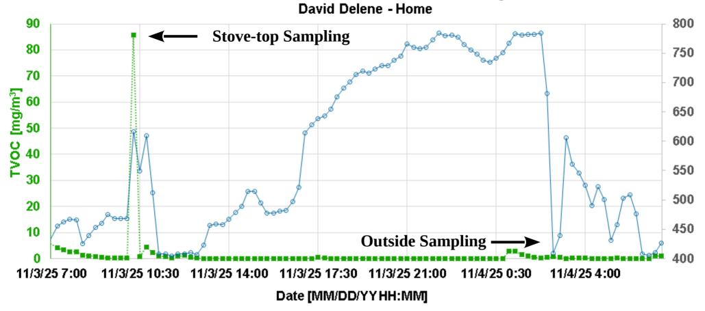
Plot showing the air quality at David Delene's home obtained with a Breathe Airmonitor Plus device. Note that after the Outside Sampling, the device was place next to open windows.
