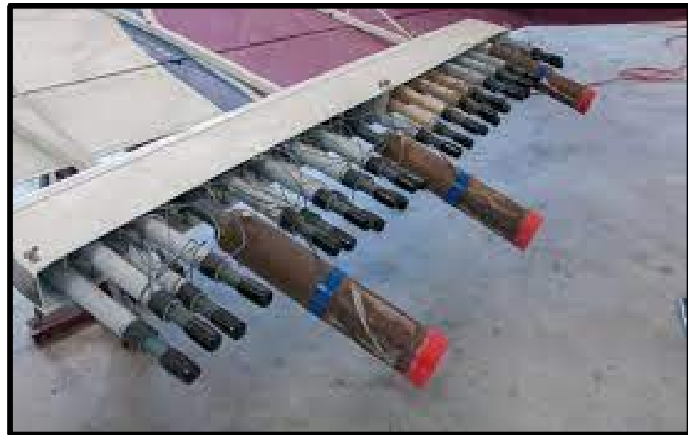
Image showing unused hygroscopic flares (left) and a three hygroscopic flares installed, along with AgI flares, on an aircraft seeding rack (right).
