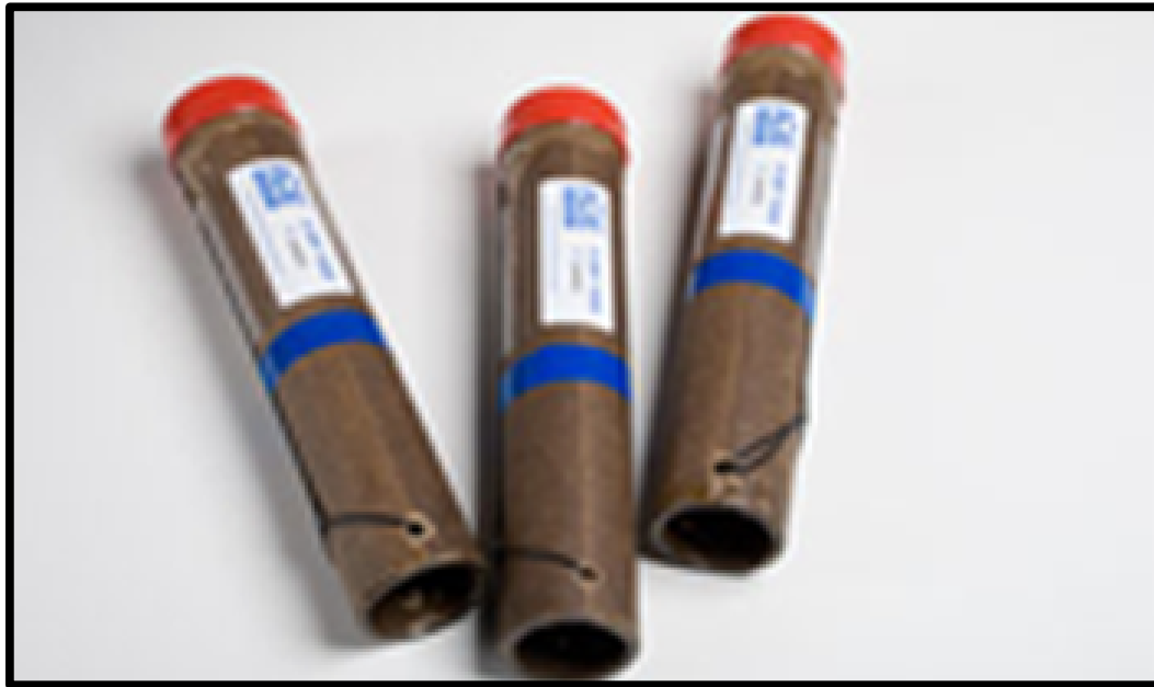
Image showing unused hygroscopic flares (left) and a three hygroscopic flares installed, along with AgI flares, on an aircraft seeding rack (right).
