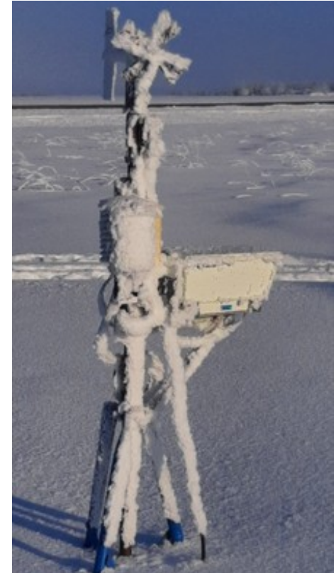
Right: Images showing ice on the TIMMS after fog event taken on in March 24 2023 at Ice Crystal Engineering.
