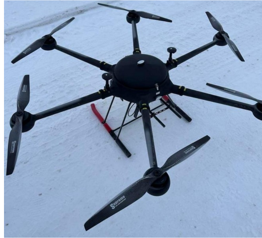
Image showing the hexacopter manufacturer by Botlink, which has a 1,620 mm diameter, 25 kg maximum takeoff weight (up to 6 kg payload), and 28 min flight duration.
