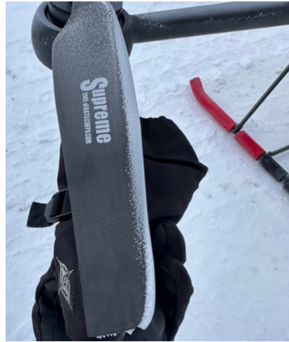
Left: Images showing ice on plates of octocopter UAS after a super-cooled fog flight in March 2023 at Ice Crystal Engineering.
