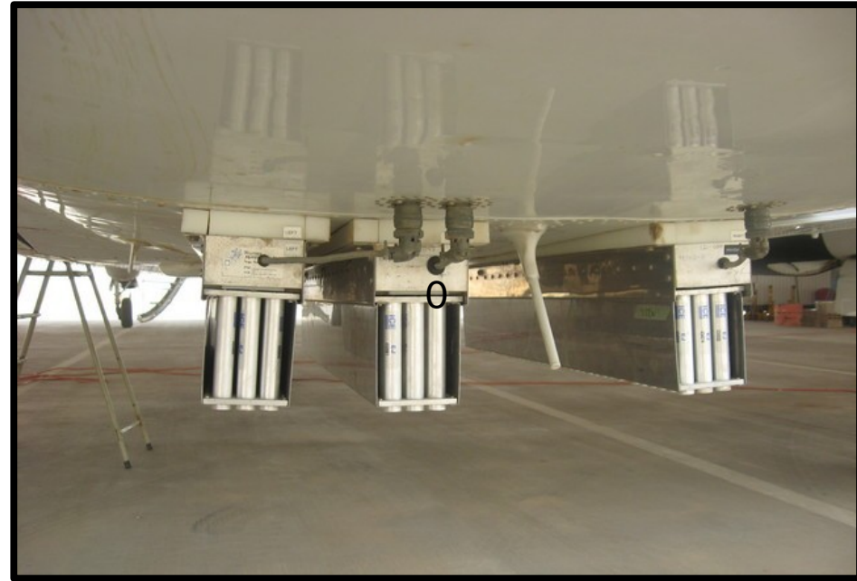
Image showing ejectable flare racks on bottom of aircraft fuselage.
