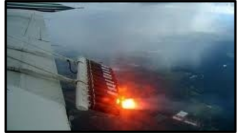
Image showing end burners (top) and burning hygroscopic flare.
