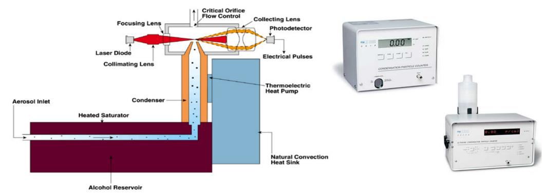
Alcohol vapor condenses onto particles which create droplets large enough to be detected one at a time by an optical particle counter. Upon entering the instrument, the air sample passes through a saturation block where alcohol evaporates saturating the flow. The air sample next enters a condenser tube which cools the air sample. Cooling of the air sample creates a supersaturated environment and the alcohol condenses onto particles, regardless of particle composition.
