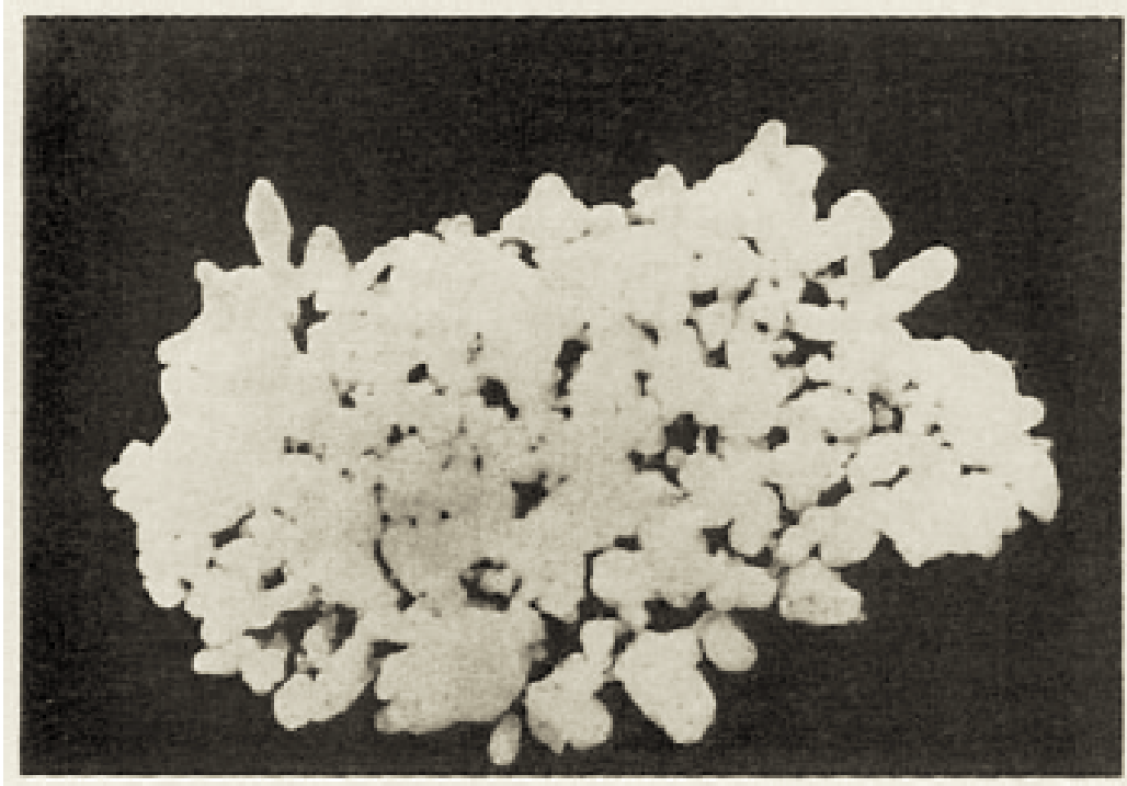
FIG. 3. Electron microscope photograph of typical AgI powder particle. Long dimension approximately 1.45\ \mu .
