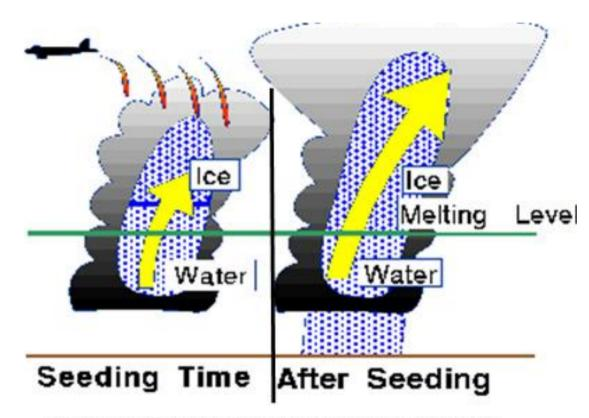
Diagram of the seeding of the upper part of a cloud by airplane, after which more rain is hoped to develop (graphic: NOAA Hurricane Research Division).
