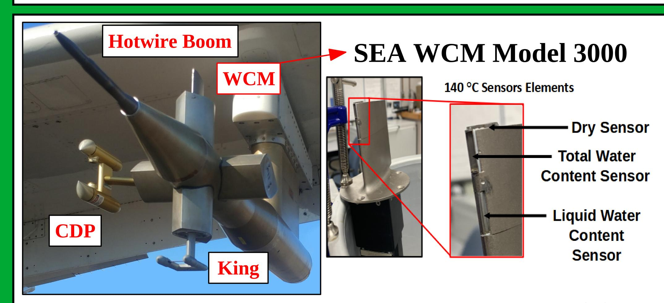
Image showing instruments on the NASA P-3 Research Aircraft for the IMPACTS 2022 field project. The Hotwire Boom has the Cloud Droplet Probe (CDP), King Probe, and Water Content Measurement (WCM) Probe.
