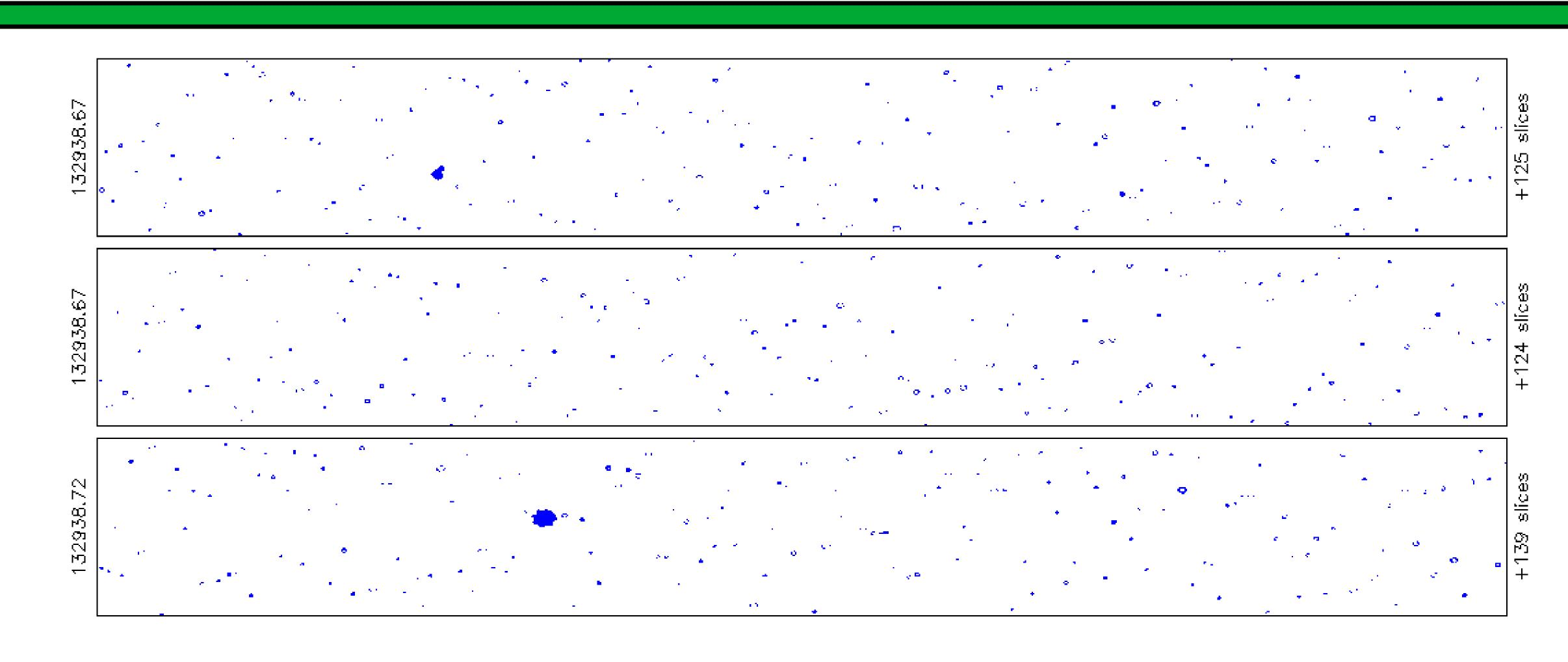
Plot showing LWC during a segment of the 19 February 2022 science flight, and corresponding images from the vertical channel of the 2D-S. The total of the y-axis for each image buffer is 1,280 µm. Note that the images show mostly small (< 50 µm) liquid water droplets, with a few lager droplets. The King, WCM, and CDP all detect liquid droplets; however, due to different upper size limits, the instruments have different LWC amounts.
