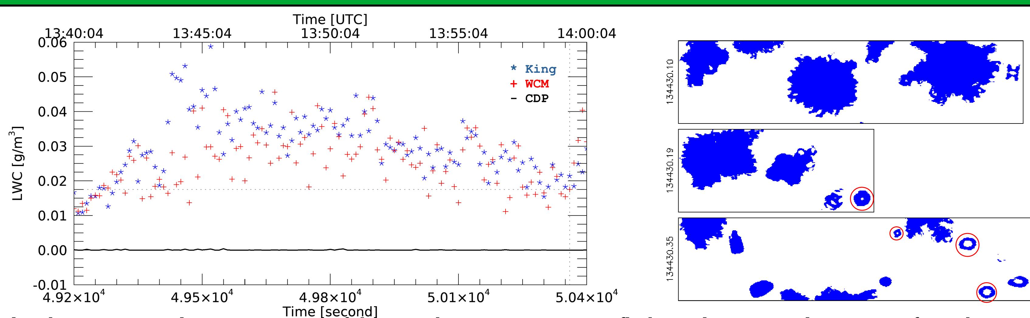
Plot showing LWC during a segment of the 19 February 2022 science flight, and corresponding images from the vertical channel of the 2D-S. The total of the y-axis for each image buffer is 1,280  $\mu$ m. Note that the images show no small (< 50  $\mu$ m) liquid water droplets, some larger (~ 150  $\mu$ m) droplets (red circles), and large ice particle. Hence, the CDP measure no LWC, while the King and WCM measure a small amount of LWC.
